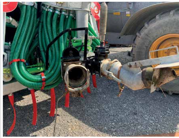
EXISTING FILL POINTS AND SPLASH PLATE RETAINED
